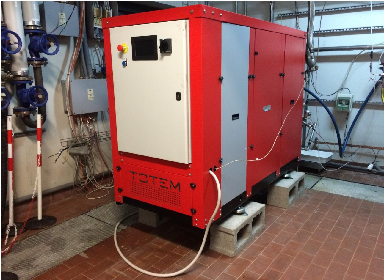
Figure 1. TOTEM 10 under testing in the Laboratory of Micro-Cogeneration at Politecnico di Milano.
