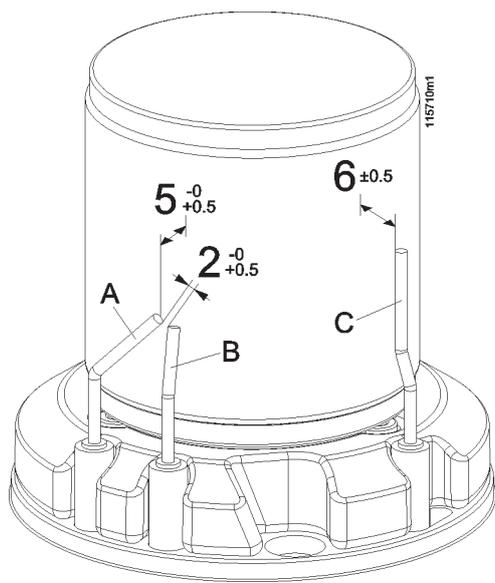
Figure 8-3 – Positioning the electrodes on the burner
