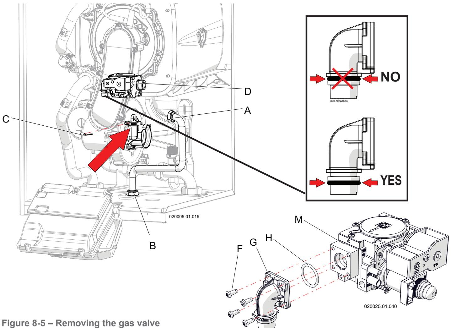
Figure 8-5 – Removing the gas valve
