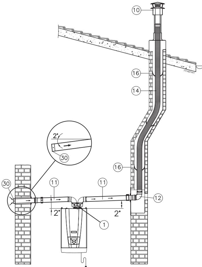
Figure 5-17 – Example of "80/80 PP system" installation
