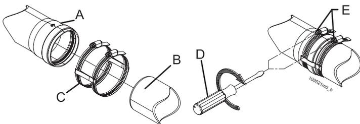
Figure 5-15 – Fixing the outlet and intake pipes
