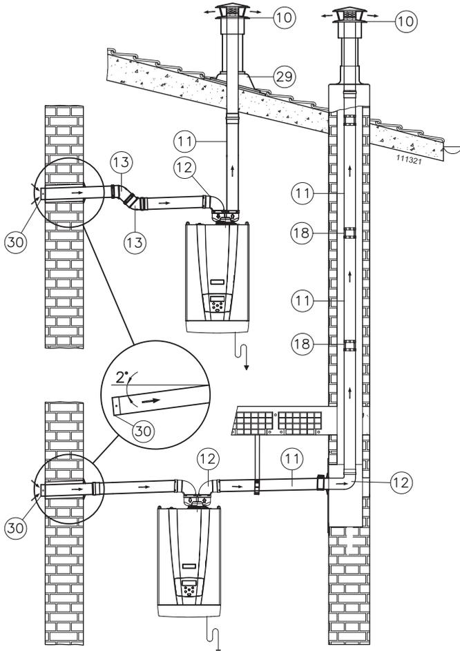
Figure 5-16 – Example of "80/80 PP system" installation
