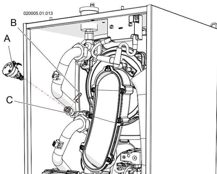
Figure 8-13 – Removing the central heating circuit pressure sensor
