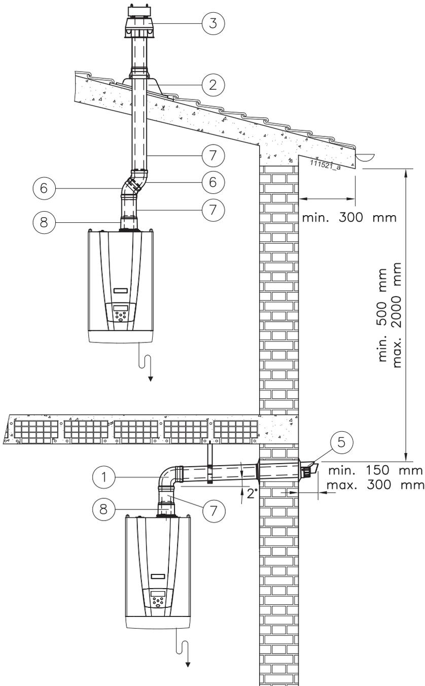
Figure 5-21 – Examples of coaxial pipe installation
