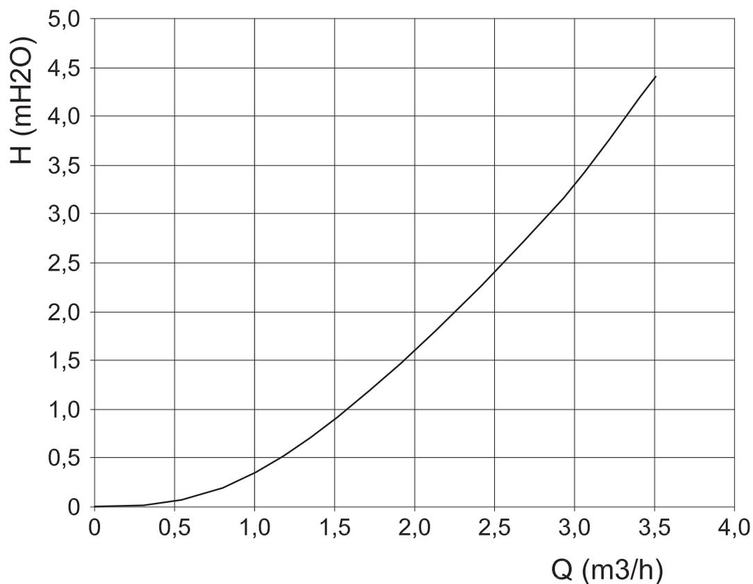
Figure 4-3 - Hydraulic resistances of MYDENS "A" boiler
