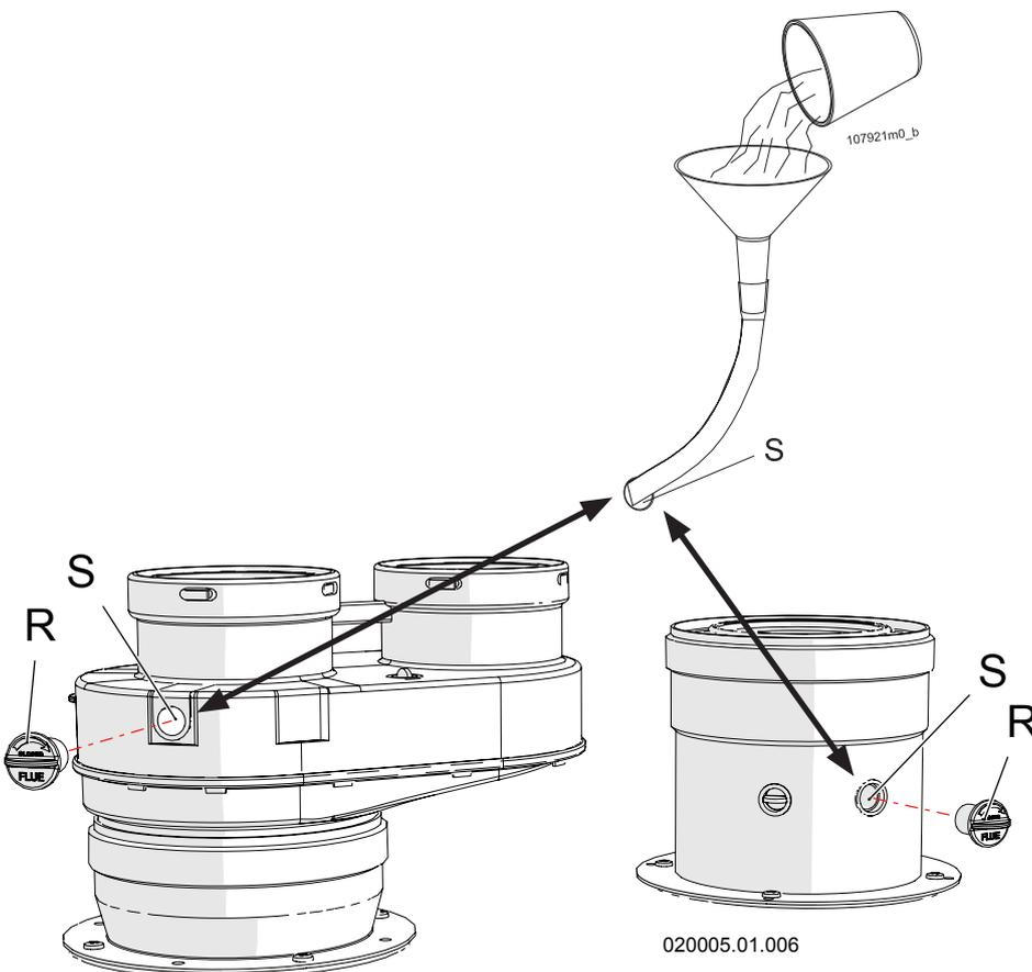
Figure 6-1 – Filling the condensate drain siphon
