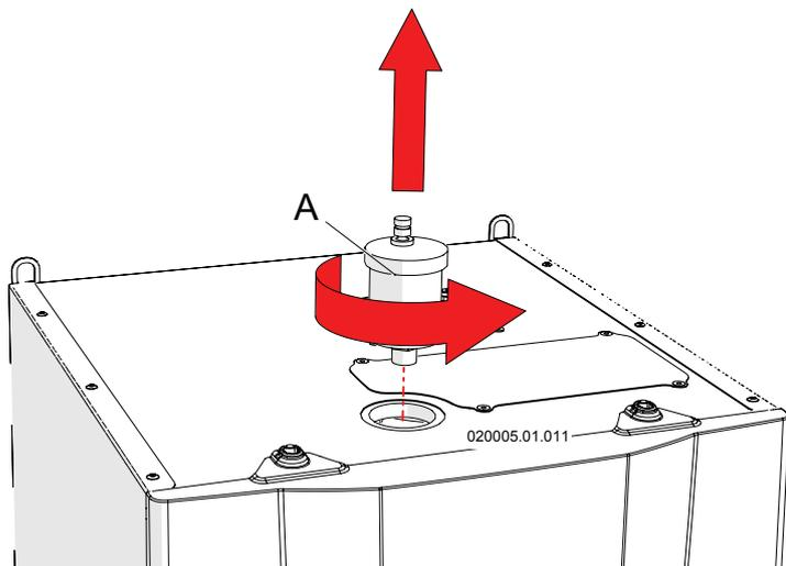
Figure 8-11 – Removing the air vent valve
