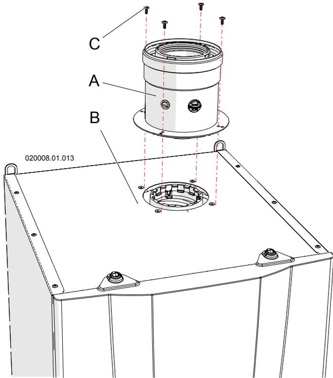
Figure 5-18 – Installation of vertical coaxial system
