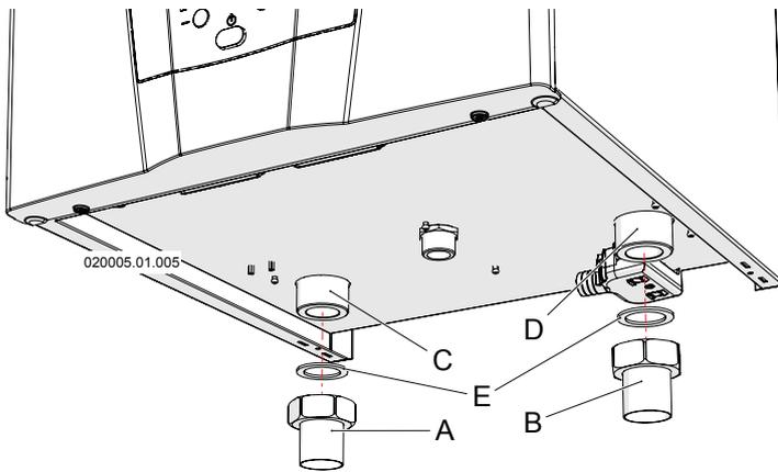
Figure 5-5 – Water connections
