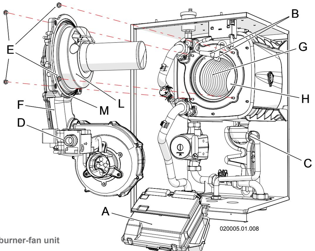
Figure 8-2 – Removing the burner-fan unit
