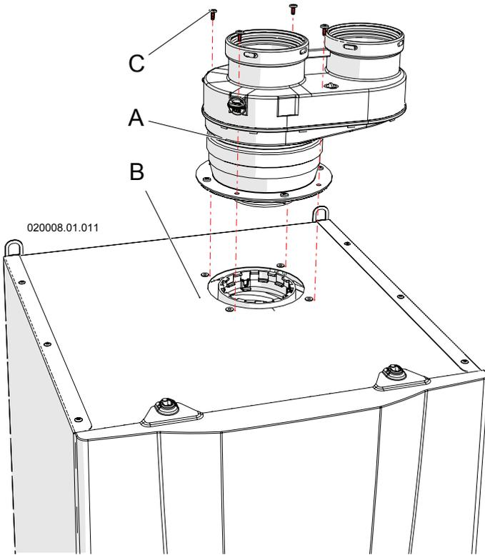
Figure 5-13 – Installing the "Split 80/80PP" system
