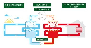
So long as the outside air temperature is above -20°C heat can be drawn out of the surrounding air to be transferred to a building's heating or hot water circuit. The UK's relatively mild winter temperatures help ensure a properly installed ASHP system can achieve excellent levels of efficiency and performance throughout the year.
