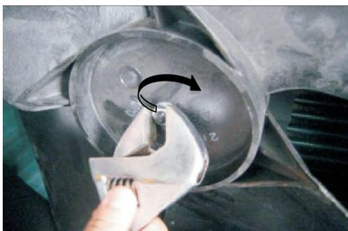
Figure 9-11 Remove the screw of fan
