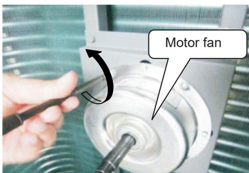
Figure 9-13 Remove the screws of the motor
