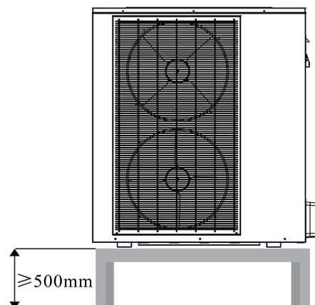
Figure 5-8 - Installation on a raised floor
