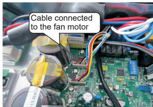
Figure 9-14 Disconnect the cable to the fan motor
