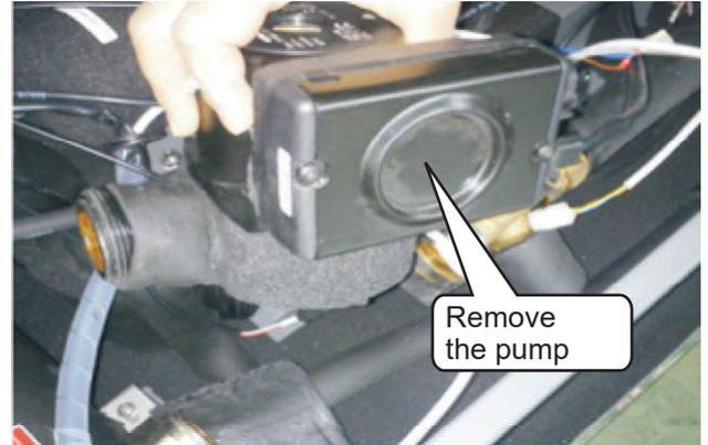
Figure 9-5 Pump removal
