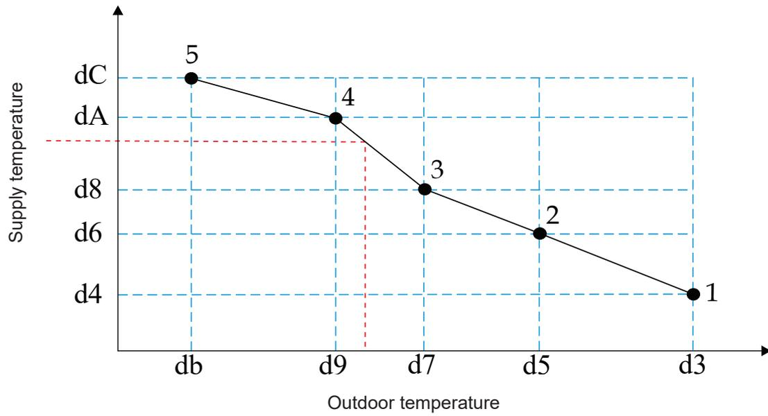
☞ In this example graph you can see how the Parameters from “d3” to “dC” (section 7.4) act on the outdoor reset and how a supply temperature is calculated as a function of the outdoor temperature.
