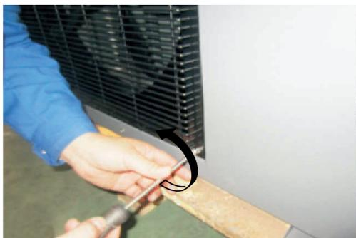
Figure 9-9 Screw of fan protection grid
