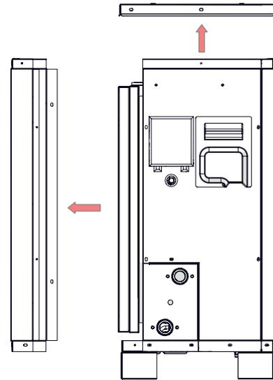
Figure 5-13 - Remove the upper and front cover
