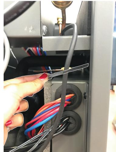
Figure 5-14 - Remove, from the inside appliance, the display cable
