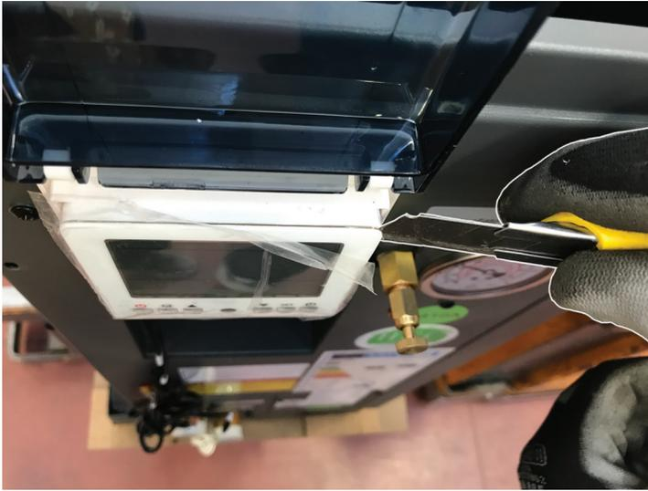
Figure 5-11 - Removal the front of the display
