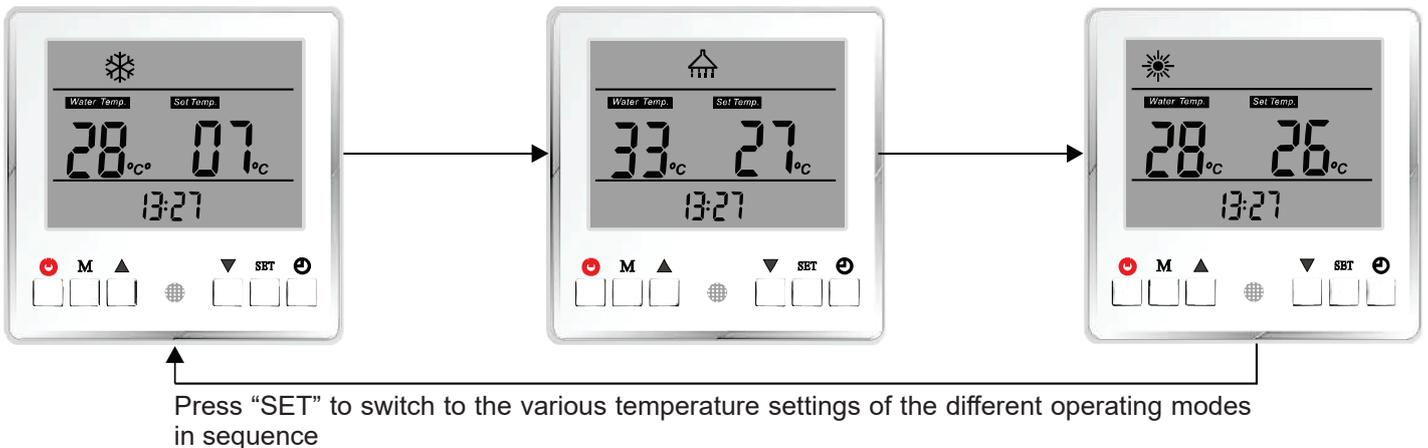
Figure 7-7 - Setting the setpoint temperature
