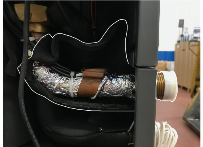
Figure 5-18 - Thermal insulation removal and access the sensors
