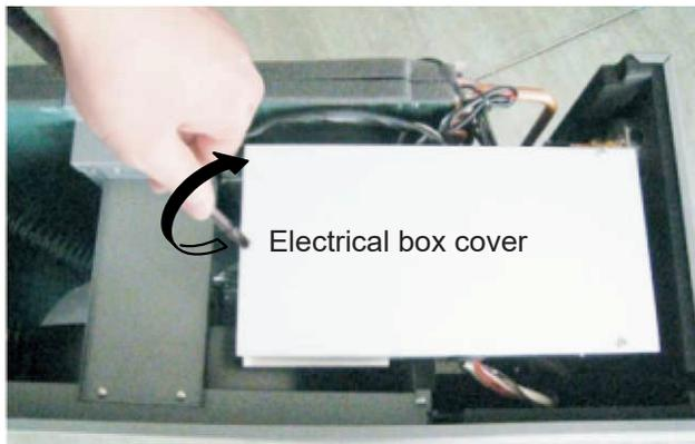
Figure 9-7 Remove the electrical box cover
