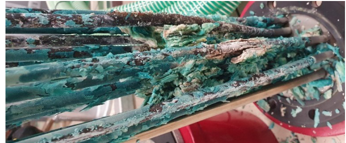
Scale collected in the bundle of an immersion heater
