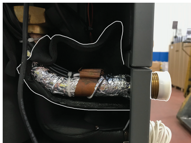
Figure 5-15 - Thermal insulation removal and access the sensors
