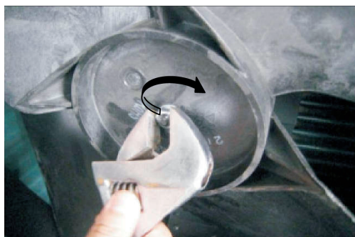
Figure 9-10 Remove the screw of fan
