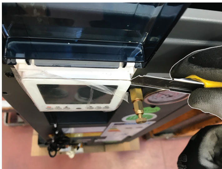
Figure 5-10 - Removal the front of the display
