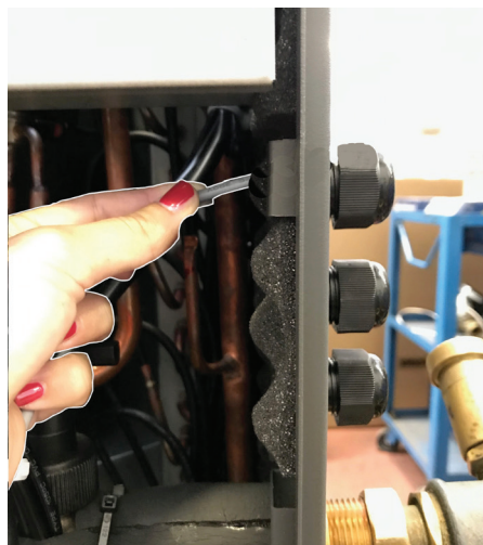
Figure 5-12 - Remove, from the inside appliance, the display cable
