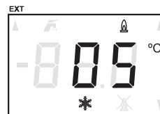
Fig. Frost protection is activated
