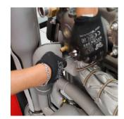
Remove the exhaust manifold.
