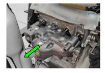
Remove the metal seal from the water-cooled exhaust manifold.
