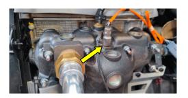
Disconnect the lambda sensor connector on the bottom of the catalytic converter.
