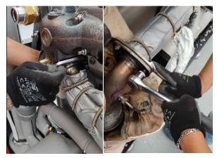
Remove the exhaust gas line pipe.
