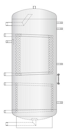
The Adveco ATSx range of stainless steel hot water tanks serve as buffer vessels and indirect hot water calorifiers suitable for use with high pressure applications.
