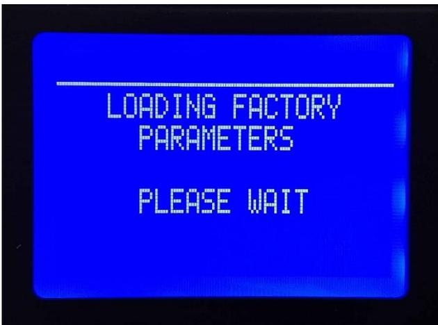
Loading the parameters usually takes ≈1 minute, after which the information appears that the parameters have been successfully written into the working memory, the CPU is quickly reset and is ready to work:
