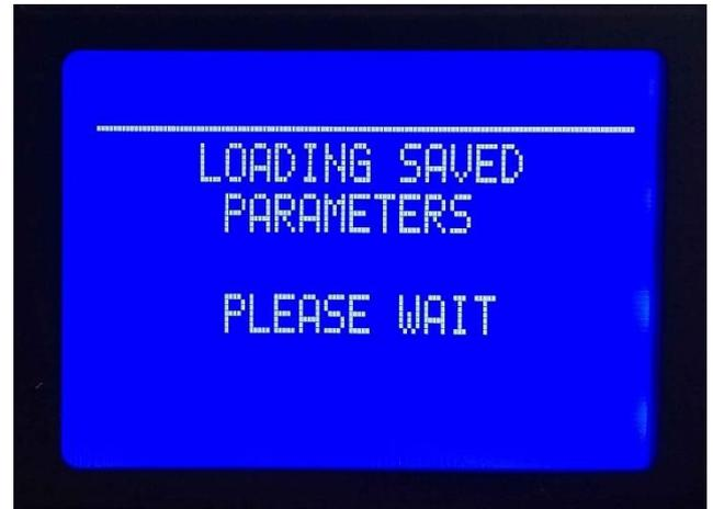
Loading the parameters usually takes  $\approx 1$  minute, after which the information appears that the parameters have been successfully written into the working memory, the CPU is quickly reset and is ready to work
